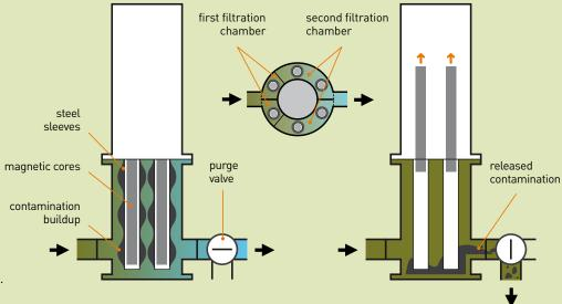
**In use** Contamination is attracted to the sleeve of the cores. Cleaned fluid is recirculated.
