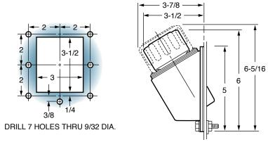
Where top surfaces are not available for locating a filler port, this unit mounts on vertical tank walls. The housing is tough, glass-reinforced nylon. It's only available with a 3-in. deep basket (and optional inner guard). The only other options are the 3-in. dipstick, the lockable cap, and powder coated cap.
