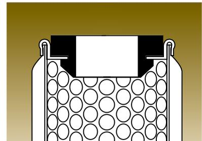
Flow Ezy seals are generally not glued onto the cartridge ends as is commonly done. Instead, they are specially shaped to hold on place mechanically, like a grommet. There is little chance they will be dislodged and lost in handling. They are made in different thicknesses to provide seven different standard overall element lengths.
