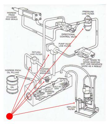
5 areas of filtration placement in a fluid power system
