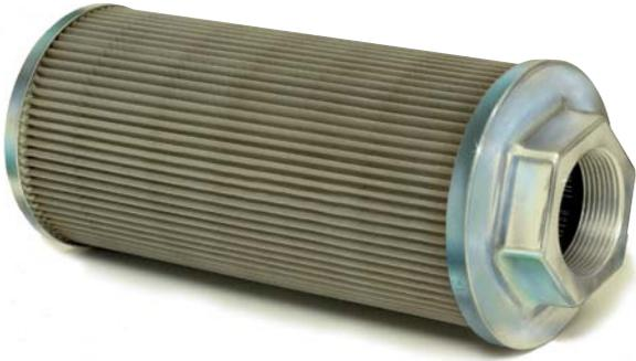
**Sump strainers are placed in the hydraulic tank below the minimum fluid level to keep large contaminants from being ingested by the pump. This strainer is available with a built-in bypass relief valve to prevent staving the pump during startup if the strainer becomes clogged.**
