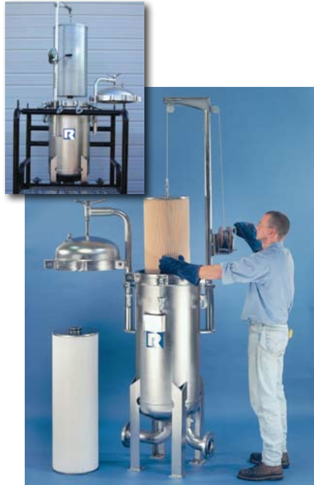
Extra large cartridges hold more contaminate.
